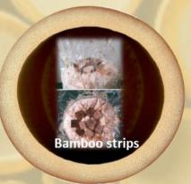
The rate of growth of the fungus are monitored over a period of time. The effectiveness of the preservation can be observed and compared by the growth of the fungus and the weight loss of the bamboo strips.
