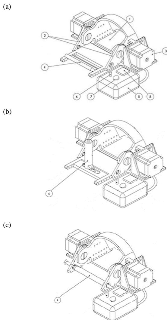
**Fig. 2** Illustrated an embodiment of the Wrist-T device. The details of hand support include a). palm rest and finger rest; b). vertical hand grip stand; and c). horizontal hand grip stand. Notes: Description of the reference numerals used in the accompanying drawings according to the WRist-T device; (1) channel; (2) platform arm; (3) motor; (4) hand support; (5) controller; (6) toggle switch; (7) power button; (8) LCD display.
