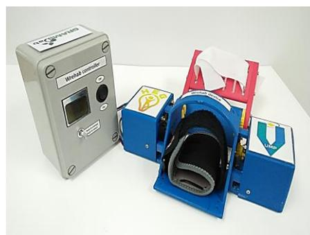
Fig. 5 The structure of the wrist rehabilitation therapy (WRist-T) device.
